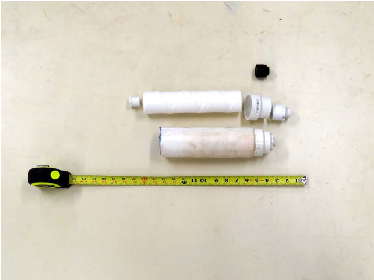
Figure 2. Black original Harbor Freight cap, components for making new filter and finished filter.
